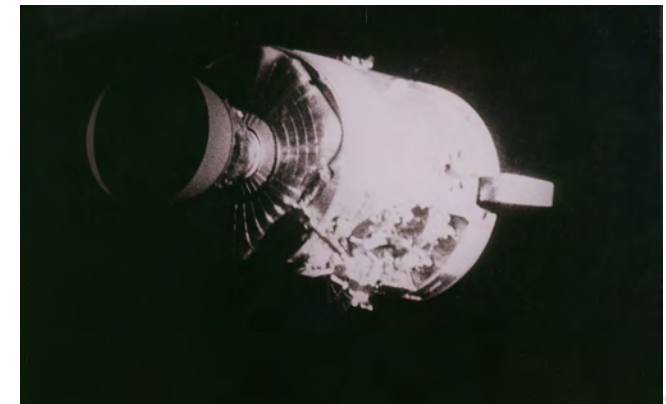
Damaged Apollo 13 Service Module. Image credit: NASA
